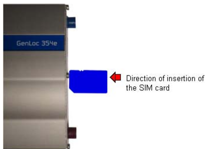
Figure 38 : Installation of the modem
