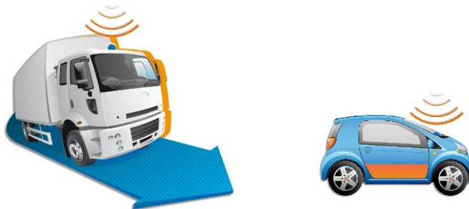
Figure 35 : Installation of GNSS antenna not recommended
