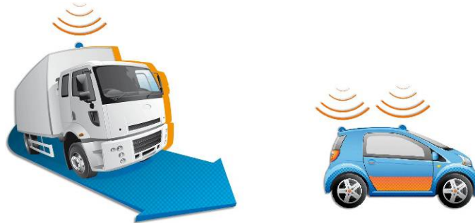
Figure 34 : Recommended installation of GNSS antenna
