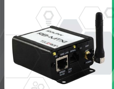
The RBMTX-Lx2 is a small modem made for wireless m2m applications. It is a compact device with all the standard interfaces and configurable GPIOs powered by Telit LE910 embedded engine. Supporting GPRS/EDGE/UMTS/HSPA+/LTE it is dedicated for users seeking for easy and the fastest mobile Internet access. Internet connection is easily available and configurable via internet browser without any need of installing software or drivers for the device.
