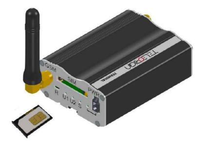
Router is available with one or two SIM card slots. To insert the second SIM card please unscrew one of the routers panel, eject PCB board and put the SIM into internal SIM holder.
