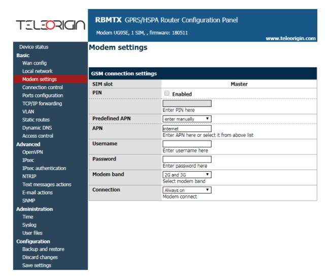
To enter the PIN for SIM card you need to mark "Enabled" field and then fill the field below with correct PIN. Please note that outgoing calls are made always on MASTER SIM card.
