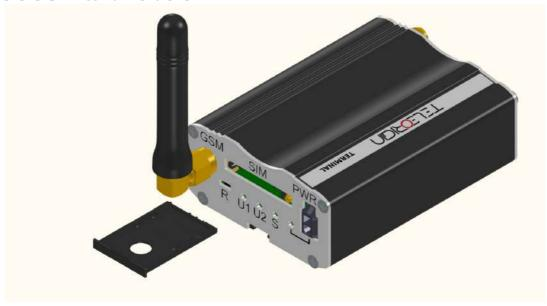
One SIM card holder is placed in front panel of RBMTX-Lite and the second one is located inside the device. To insert SIM card into the extractable holder **push yellow button and take SIM drawer out** as show in the picture and place SIM card. To operate the module in a GSM network, it is necessary to insert at least one active SIM card.
