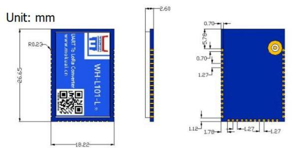
Figure 1 Dimension diagram
