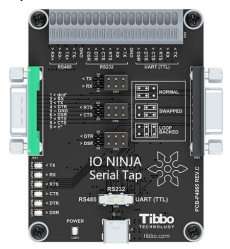
IO NINJA Serial Tap is an affordable serial sniffer that can monitor RS232, RS485, and TTL-level UART communications. The Tap connects to your PC via a USB cable and is compatible with IO Ninja terminal/sniffer software for Windows.
