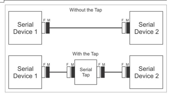
Of course, DB9 genders on the serial devices may differ from the above example, and so your serial arrangement may be different. To aid you in the "wedging process," each Serial Tap comes with two DB9 gender changers.
