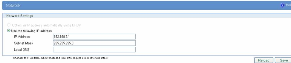
Figure 56 - Network configuration page for GWR-I Router 2
