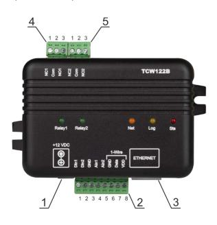
**Connector 1** – Power - 2.1x5.5mm connector, central positive
