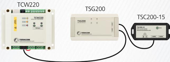
**Attention!** Only one sensor TSG200 can be connected to a controller. It should be placed on 10 m maximum from the controller.
