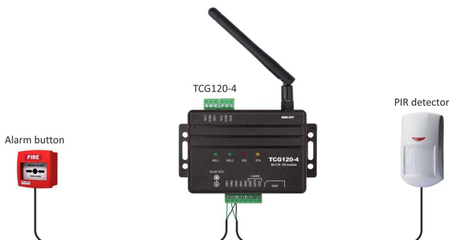
The maximum cable length for a digital input should be up to 30 meters.
