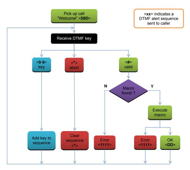
The "welcome" alert will be re-sent to the caller after 10 seconds of inactivity. The call will automatically hang-up after 60 seconds of inactivity.
