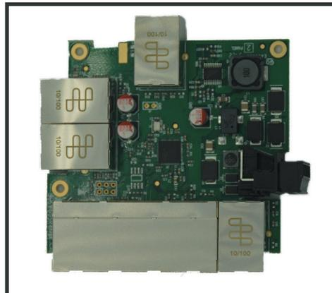
Embedded format, takes up minimal space, with mounting holes are connected to Functional Earth
