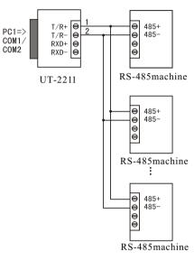
3.UT-2211 half-duplex communication connect between interface converter
