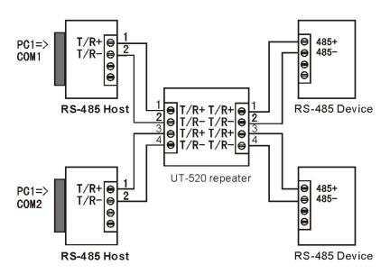
2. RS-485 point-to-multipoint / 2-line half duplex relay communication
