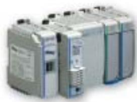
SST AS-Interface module connects your Allen-Bradley CompactLogix / MicroLogix 1500 controller to AS-Interface network.
