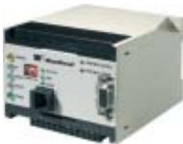
The Direct-Link Profibus to Serial or Ethernet gateway supports local communications through an RS232/RS485 serial port, a 10/100 Base-T Ethernet port and a Profibus port. Network data mapping is used to automatically transfer data between devices connected to the gateway. A simple software application is provided to create the routing tables and data mappings.
