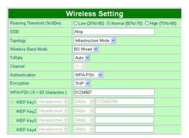
Fig 26. WPA-PSK Authorization and TKIP Encryption
