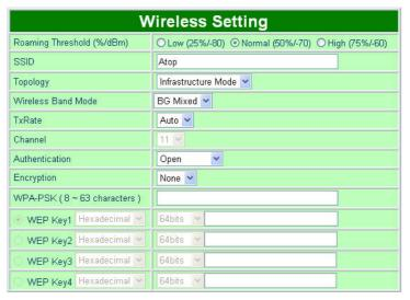
Fig 24. Open Authorization and no Encryption
