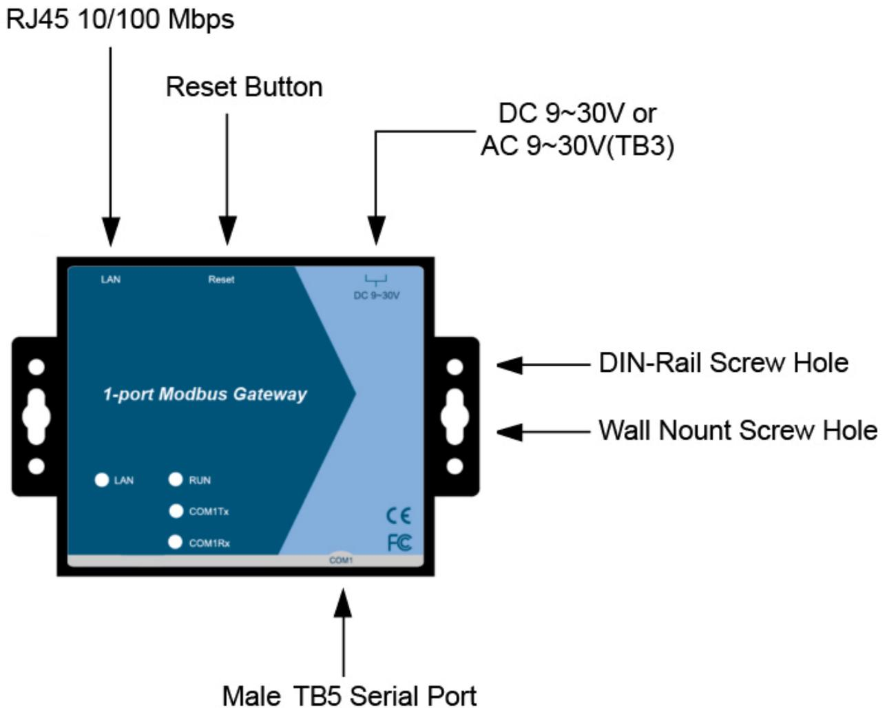
Figure 2.2 MB5001C-Sis interfaces
