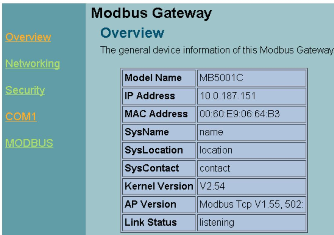
The screenshot shows a web interface for a Modbus Gateway. On the left is a navigation menu with links for Overview, Networking, Security, COM1, and MODBUS. The main content area is titled "Modbus Gateway Overview" and contains a table of device information.
