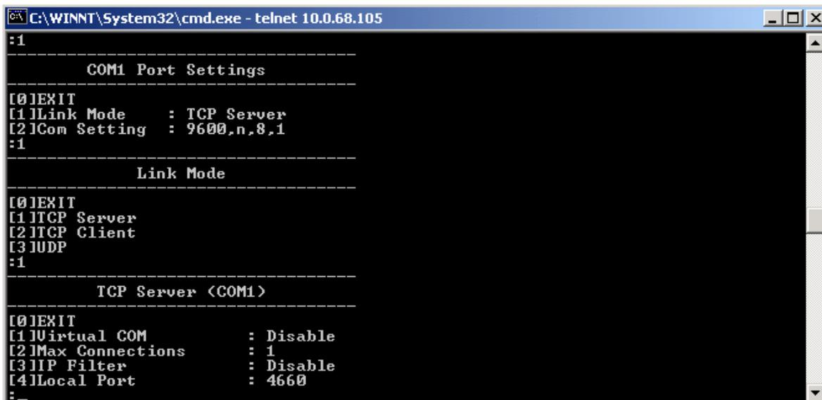
Figure 3.15 TCP Server for Link mode
