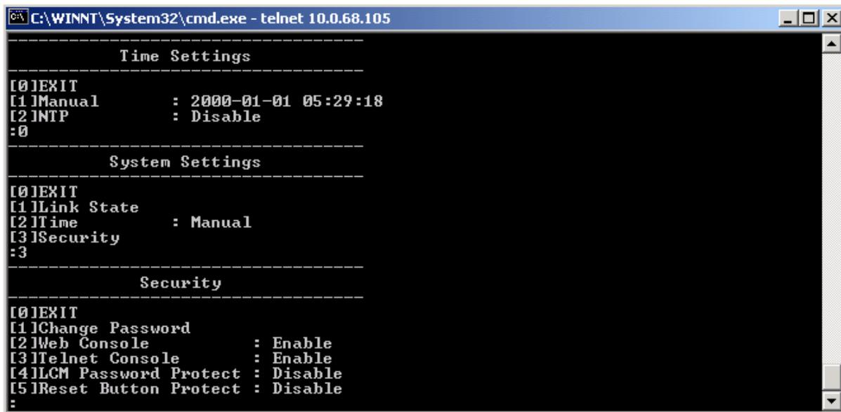
Figure 3.27 Security Settings by Telnet
