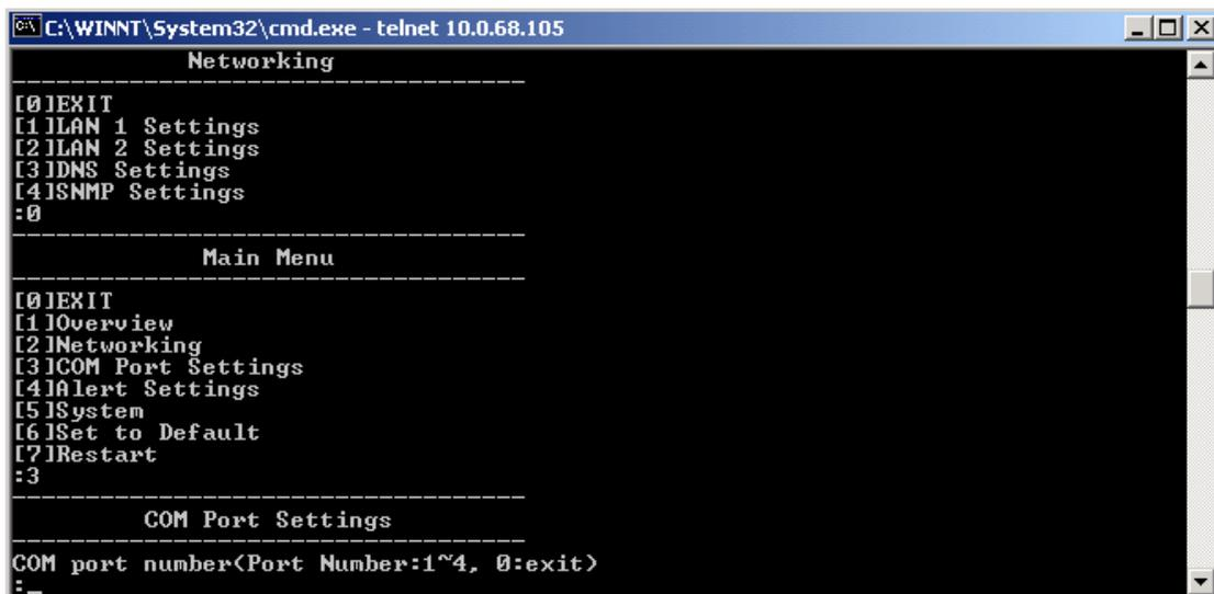
Figure 3.14 Select COM Port from Serial Settings by Telnet
