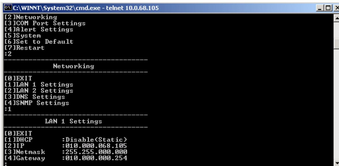
Figure 3.8 LAN 1 Settings by Telnet
