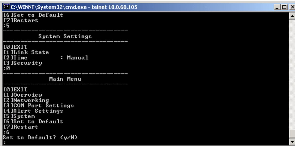
Figure 3.28 Restore Factory Default by Telnet
