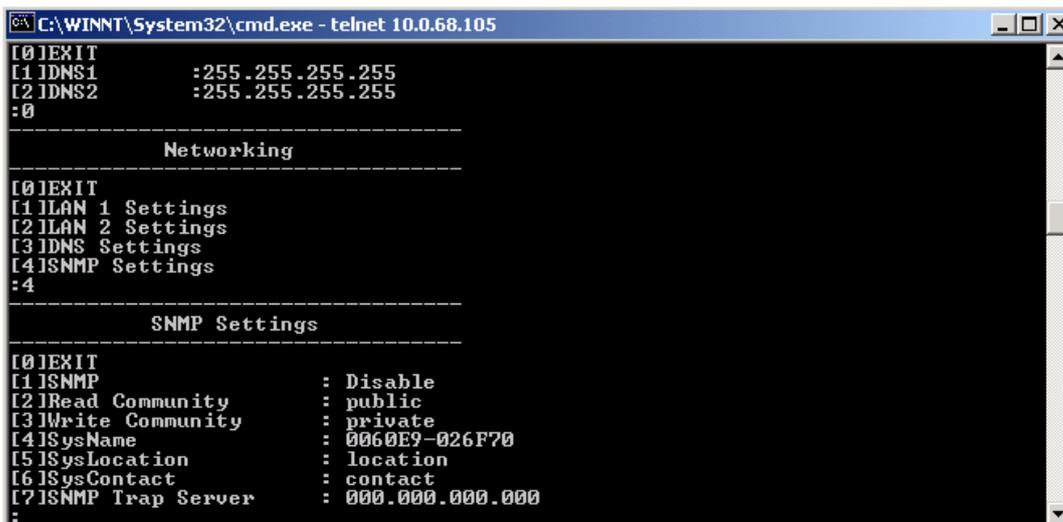
Figure 3.12 SNMP Settings by Telnet
