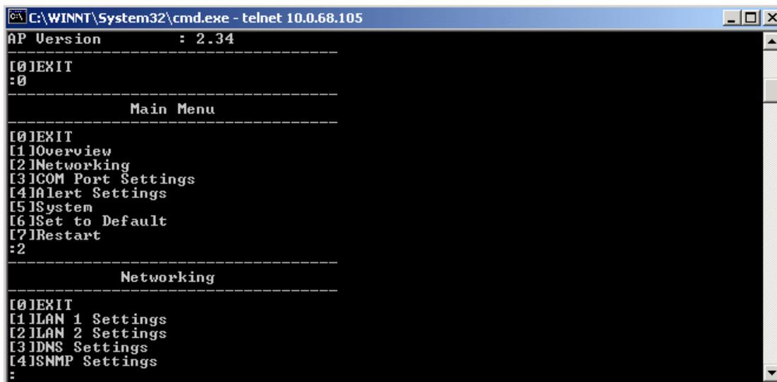
Figure 3.7 Network Settings by Telnet
