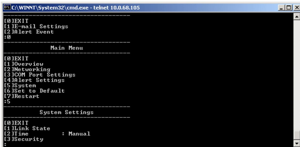
Figure 3.24 Security settings by Telnet
