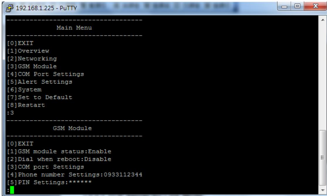
Figure 3.12 GSM Module Settings by Telnet
