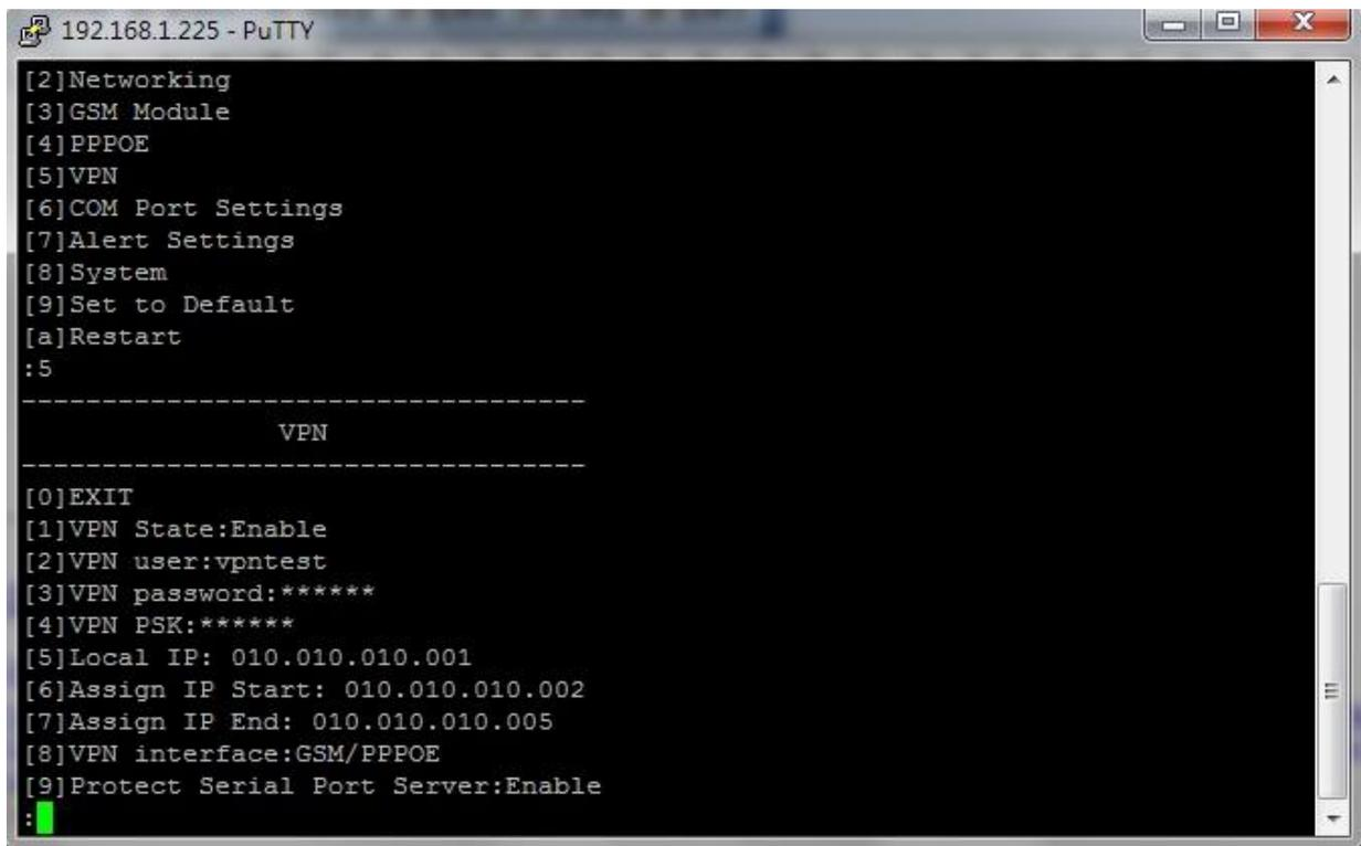
Figure 3.14 VPN Settings by Telnet
