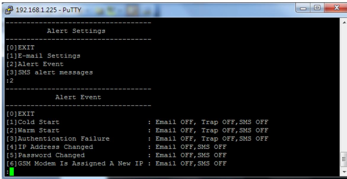
Figure 3.22 Configuring Alert Event by Telnet
