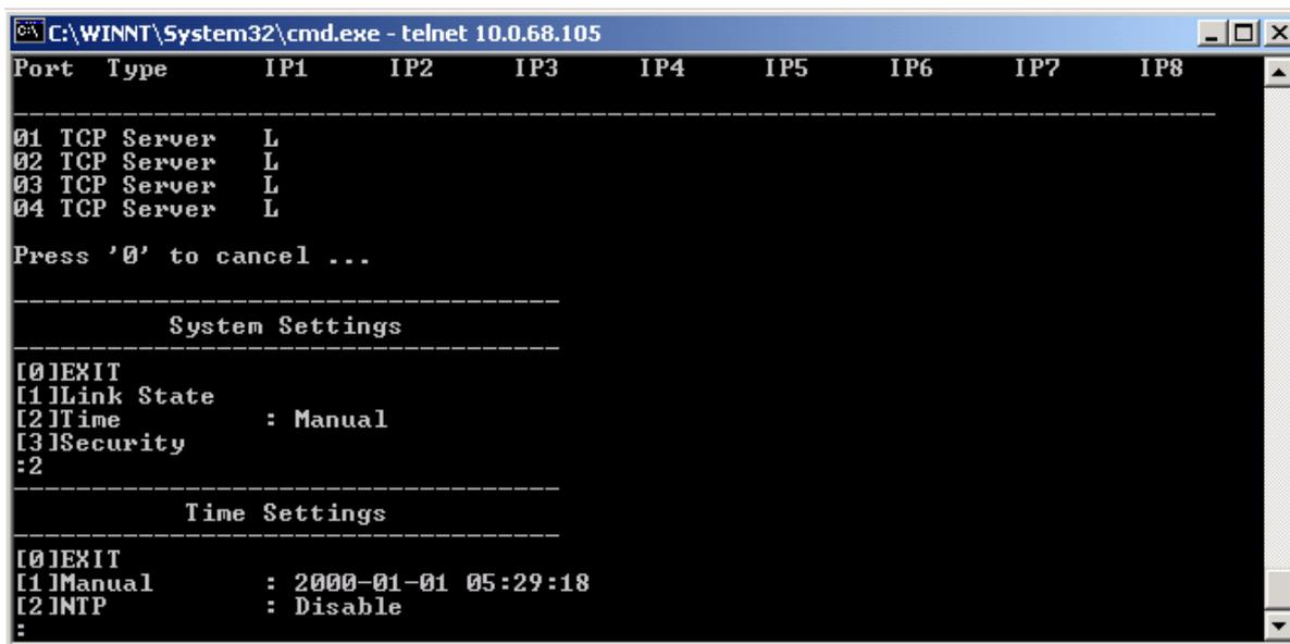
Figure 3.26 Time settings by Telnet
