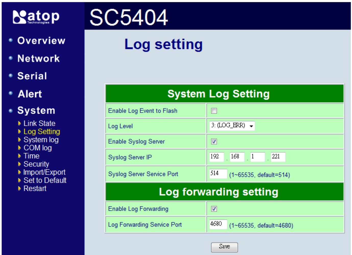
Figure 3.42 System Log Setting WebUI
