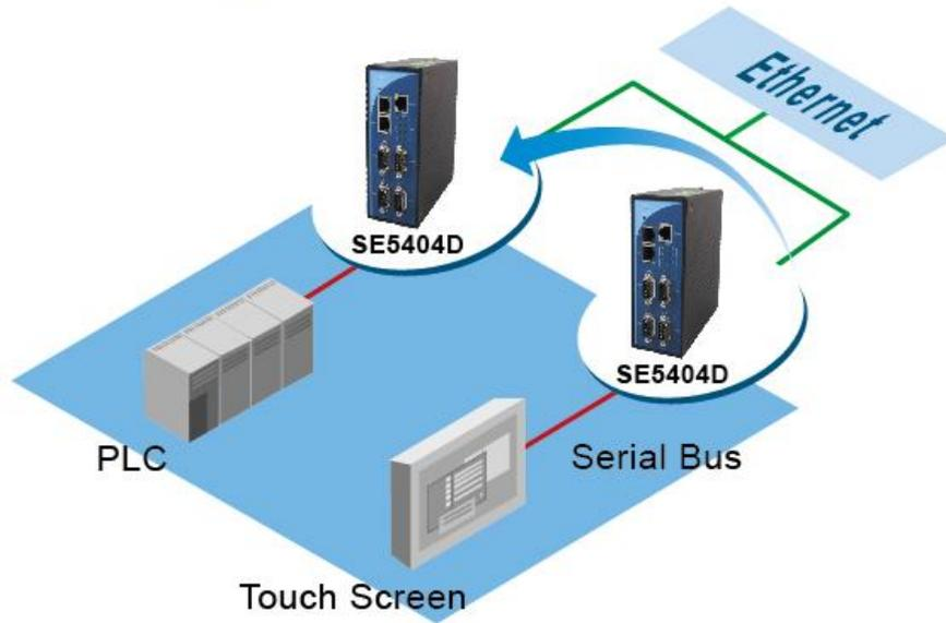
Figure 1.4 Tunneling Mode
