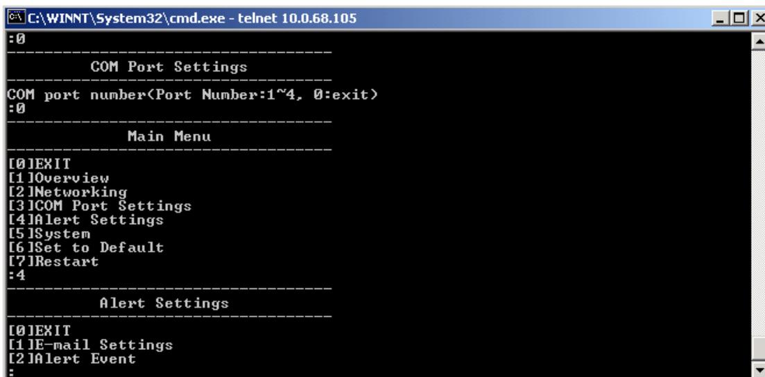
Figure 3.19 Alert Settings by Telnet
