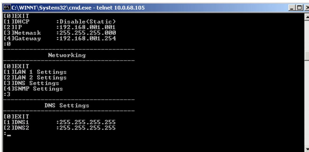
Figure 3.10 DNS Settings by Telnet
