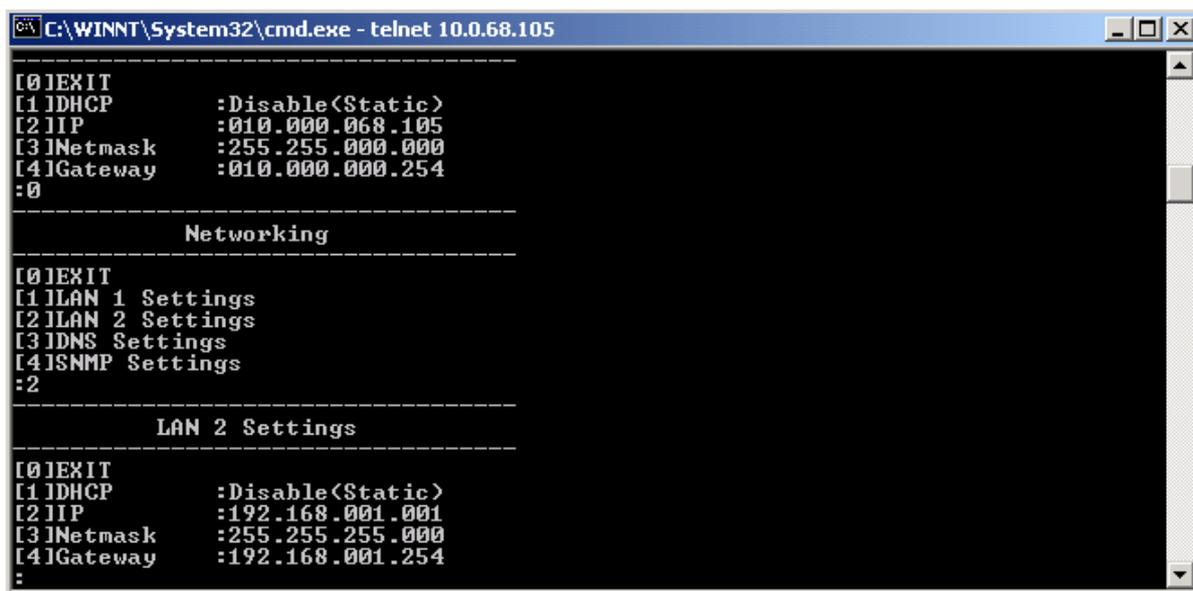
Figure 3.9 LAN 2 Settings by Telnet
