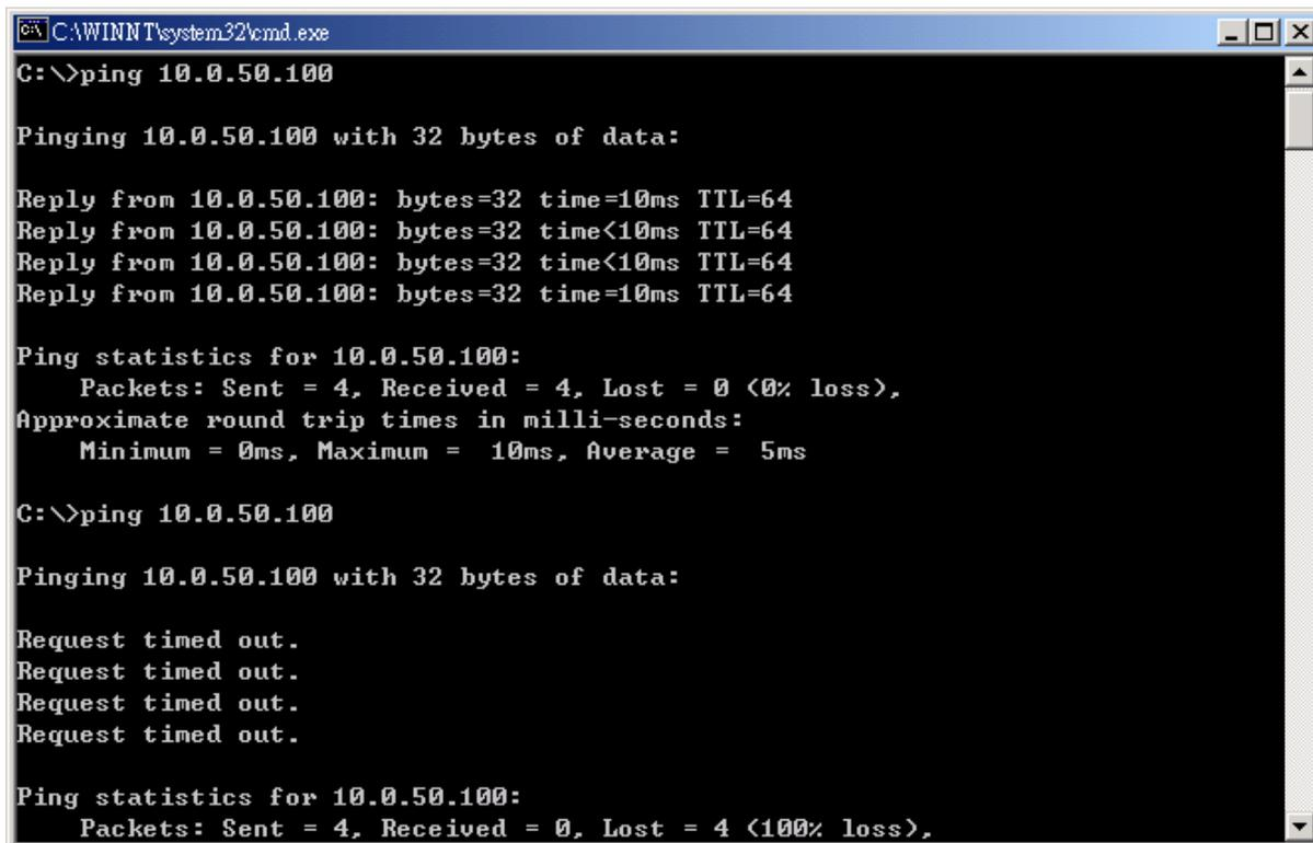
Figure 7.1 Standard TCP/IP utility ping command
