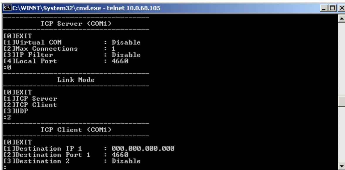
Figure 3.16 TCP Client for Link mode
